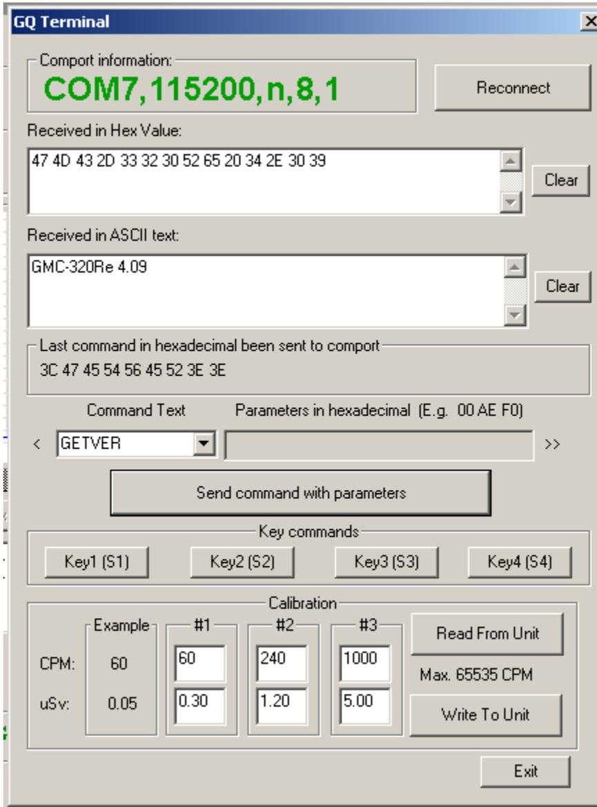
The GQ Terminal provides an immediate access interface to the GMC-500 communication protocol.
