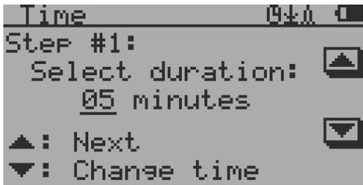
This mode can be used for comparing radiations between two samples. It can be also used for comparing food radiation to the background.
