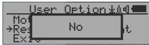
The Reset Total Count menu item let user to clear the total count on main text mode screen. This may be used before a fixed time count measurement start.
