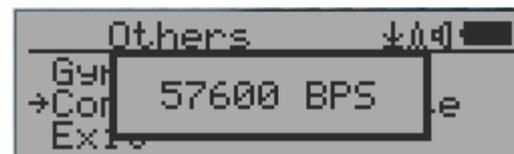
This Geiger counter serial communication baud rate is selectable from following value: 1200,2400,4800,9600,14400,19200,28800, 38400, 57600, and 115200. Press S4 key changes baud rate.
