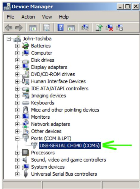
For the data viewer or the data logger software, selecting COM5 will establish the connection to the GMC-500 Geiger counter for the above example
