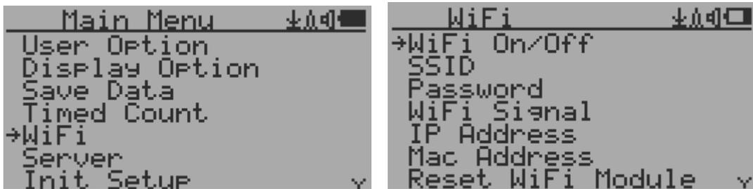
Select Wi-Fi On/Off item will turn the Wi-Fi connection On/Off
