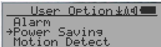
Pressing the S4 key will toggle the Power Saving mode ON and OFF.
