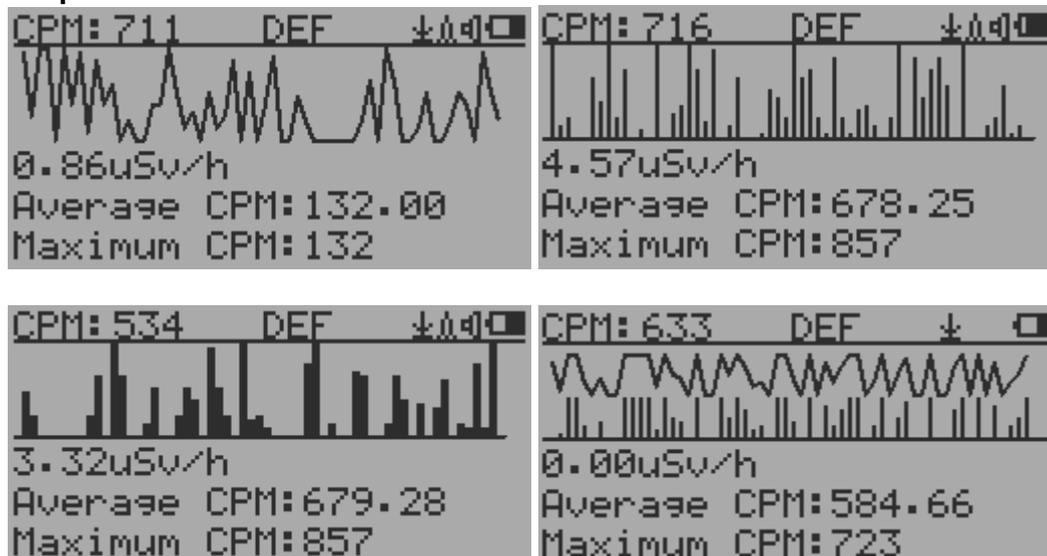
**CPM: 606** Current radiation level reading in CPM format (Counts Per Minute)
