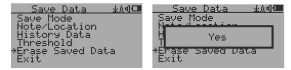
Use S2 and S3 to select Yes or No on the screen to confirm the request. After about 3 seconds with Yes confirmation, the unit will start to erase entire saved history data. It may take a few seconds to complete the task.
