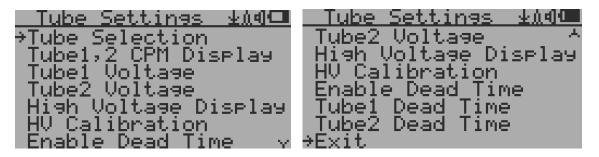
Tube Selection allow user to select the active tube: #1 high sensitivity tube, #2 high dose tube or both
