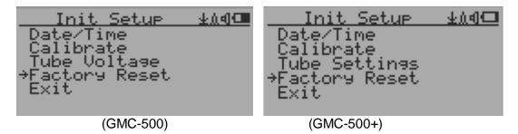
Select Factory Reset to reset the unit to the factory default settings.
