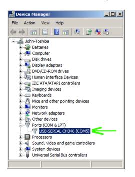
For the data viewer or the data logger software, selecting COM5 will establish the connection to the GMC-500 Geiger counter for the above example
