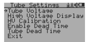
Tube Voltage: about 3 to 600V, Steps: 1 to 100, the voltage change is not in linear. High Voltage Display: Display high voltage reading in Text Mode HV Calibration: For adjusting the high voltage reading Enable Dead Time: For including tube dead time in the CPM calculation Tube Dead Time: Dead Time Value
