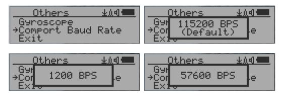
This Geiger counter serial communication baud rate is selectable from following value: 1200,2400,4800,9600,14400,19200,28800, 38400, 57600, and 115200. Press S4 key changes baud rate.
