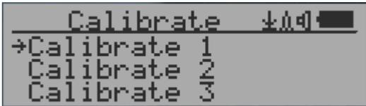
Each calibration point needs two values to be entered, the CPM value and the  $\mu\text{Sv/h}$  value. The user can enter up to three calibration points from large to high count rates.
