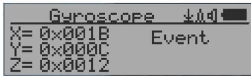
The internal digital accelerometer is able to provide real-time gyroscope data. It displays current unit X, Y, Z axis data and detected motion event. Such as single tap OR double tap.
